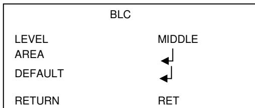
The options available for LEVEL are: middle, high, low. The function AREA allows to define dimension and position.
