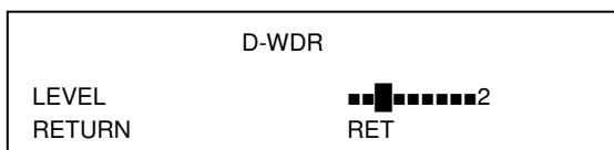
Selecting LEVEL and moving to left or right you can reduce the differences in brightness between light and dark areas.
