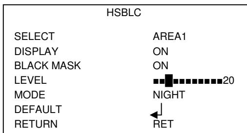
The SELECT menu provides 4 areas. For those areas set their position and size (DISPLAY), their brightness level (0 to 255) and their MODE (ALL DAY and NIGHT, which you can adjust the AGC LEVEL for) to enable the BLACK MASK . You can use the DEFAULT command to reset the previous values.
