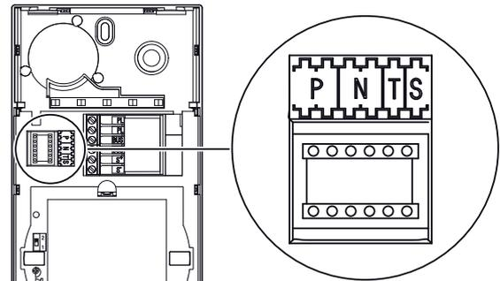
For the Classe 100 and Classe 300 internal units, the S configurator associates the entrance panel to the bell programmed in the internal unit.
