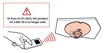
• 088230/BMSO4001: Advanced configuration tool When the sensor receives an IR command via a configuration tool, the LED blinks.
