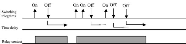
d) Delay before OFF + delay before ON
