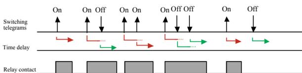
h) Delay before ON + Delay before OFF + Auto Switch OFF
