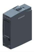
SIMATIC ET 200SP, Relay module, RQ NO 4x 120V DC..230VAC/5A ST. 4 normally open contacts, isolated contacts, packing unit: 10 pieces, fits to BU-type B0 and B1, Colour Code CC40, substitute value output, module diagnostics for: supply voltage
