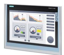
SIMATIC HMI TP1500 Comfort, Comfort Panel, touch operation, 15" widescreen TFT display, 16 million colors, PROFINET interface, MPI/PROFIBUS DP interface, 24 MB configuration memory, WEC 2013, configurable as of WinCC Comfort V14 SP1 with HSP, ambient temperature up to 50  $^{\circ}$ C (up to 55  $^{\circ}$ C with restrictions)
