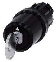
key-operated switch Siemens, 22 mm, round, plastic, lock no. SSG1, with 2 keys, 3 switch positions I>O<II, momentary contact on the left, latching on the right, actuating angle 2x45°, 10:30h/12h/13:30h, key removal O
