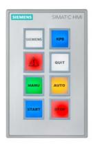
SIMATIC HMI KP8F PN, Key Panel, 8 short-stroke switches with multi-colored LEDs, PROFINET interfaces with PROFIsafe; 8 DI/DO and 2 safety DI pins, 24 V DC can be looped through parameterizable as of STEP 7 V5.5
