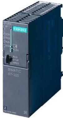
SIMATIC S7-300, CPU 312 Central processing unit with MPI, Integr. power supply 24 V DC, Work memory 32 KB, Micro Memory Card required
