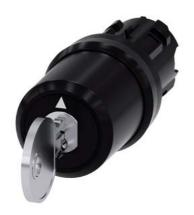
Key-operated switch BKS, 22 mm, round, plastic, lock number S1, with 2 keys, 3 switch positions I>O<II, momentary contact type, actuating angle  $2x45^\circ,\,10:30h/12h/13:30h,$  Key removal O
