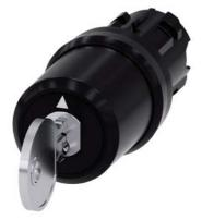
Key-operated switch BKS, 22 mm, round, plastic, lock number S1, with 2 keys, 3 switch positions I-O-II, latching, actuating angle 2x45°, 10:30h/12h/13:30h, Key removal I+O+II
