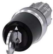
Key-operated switch IKON, 22 mm, round, metal, shiny, lock number 360012K1, with 2 keys, 3 switch positions I-O-II, latching, actuating angle 2x45°, 10:30h/12h/13:30h, Key removal I+O+II
