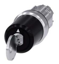
key-operated switch Siemens, 22 mm, round, metal, shiny, lock number SSG10, with 2 keys, 3 switch positions I-O-II, latching, actuating angle  $2x45^\circ,\,10:30h/12h/13:30h,$  key removal O
