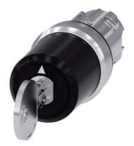
Key-operated switch BKS, 22 mm, round, metal, shiny, lock number S1, with 2 keys, 3 switch positions I>O<II, momentary contact on the left, latching on the right, actuating angle  $2x45^{\circ}$ , 10:30h/12h/13:30h, Key removal O
