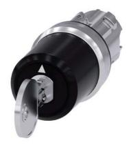
Key-operated switch BKS, 22 mm, round, metal, shiny, lock number S1, with 2 keys, 3 switch positions I-O-II, latching, actuating angle  $2x45^\circ$ , 10:30h/12h/13:30h, Key removal I+O+II
