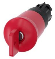
EMERGENCY STOP mushroom pushbutton, 22 mm, round, plastic, red, 40 mm, with O.M.R. lock, lock number 73037, positive latching, acc. to EN ISO 13850, key-operated release
