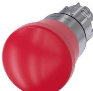
EMERGENCY STOP mushroom pushbutton, 22 mm, round, metal, shiny, red, 40 mm, positive latching, acc. to EN ISO 13850, pull-to-unlatch mechanism
