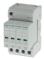
Surge arrester T2, UN 240/400 V, UC 350/264 V AC, pluggable protective module, 3+1 circuit (TN-S, TT), Width 49.2 mm
