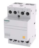
INSTA contactor with 4 NO contacts Contact for 230 V AC, 400V 40A Control 24 V AC
