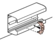
By removing the part of completion of the cover joint, that gives access simply the cover to withdraw it and facilitates the intervention in the compartment.
