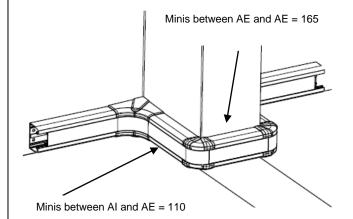
Mini dimension in mm to be respected allowing the installation of angle inter/exter: (in the case of a skirting of post for example)
