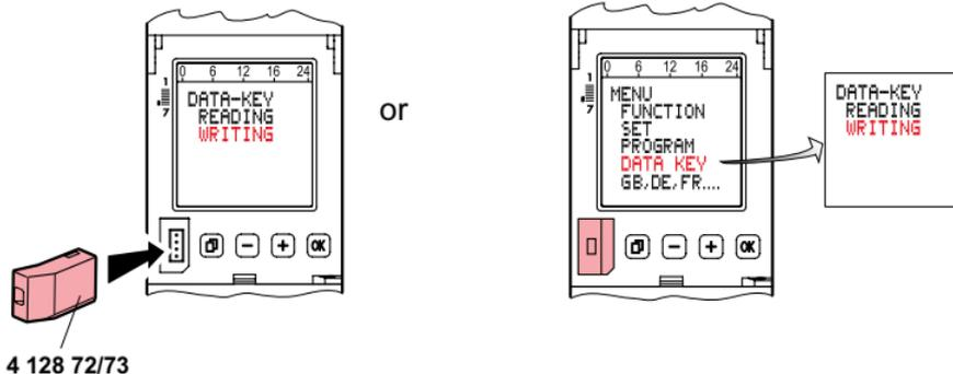
**Load the programs of the time switch on to a data key (WRITE KEY)**
