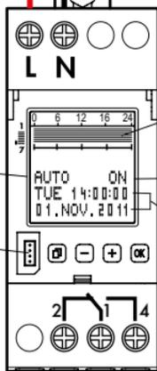
Overview of programmed switching times for the week. Resolution 0.5h
