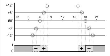
If the offset setting is in degrees the time switch switches on and off at times of equal brightness, despite the differences in twilight time lengths over the course of the year.
