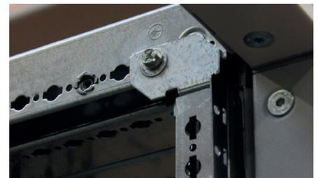
The faceplate support uprights are fixed in the first tapped hole 50 mm from the front (below the earth symbol).
