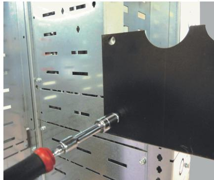
Screw in the middle panel using the eight screws supplied.
