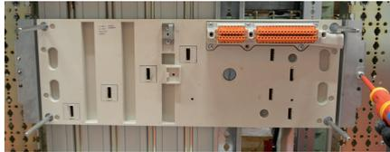
The fixed part of the VX<sup>3</sup> base is finally secured on the IS chassis uprights by using the two screws supplied (don't forget to insert the two clip-nuts in the uprights first).
