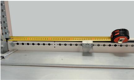
Place the top and bottom fixing lugs 375 mm from the left-hand side of the enclosure.
