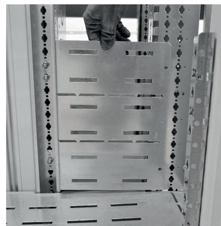
To obtain form level 3b, the part of the IS chassis not equipped with the VX<sup>3</sup> IS base must be closed at the front with 300 mm high spare compartments Cat.No 4 046 89. If necessary, they can be cut at 100 mm intervals.
