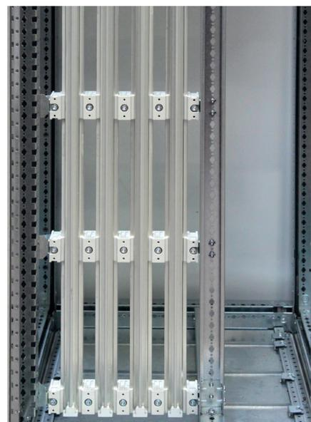
The flanges ensure the mechanical strength of the busbars on the chassis (tightening torque: 20 N·m).
