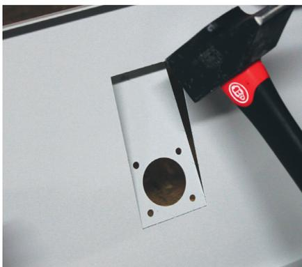
The faceplate is common to circuit breakers equipped with a rotary handle or motor-driven control. When installing a motor-driven control it will be necessary to break the specially provided cut-out.
