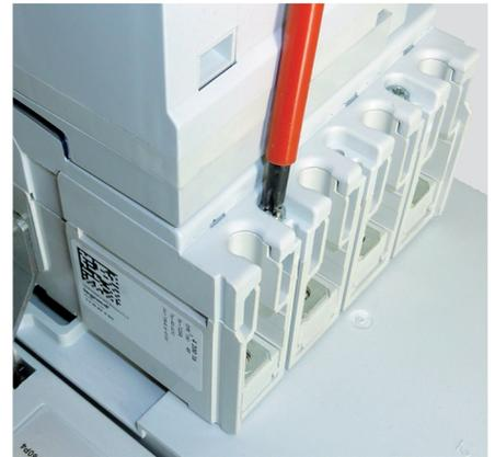
Place the appliance on the base, then secure it with the screws supplied with the circuit breaker (tightening torque 1 N·m).
