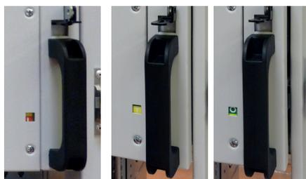
The three tray positions: "inserted", "test", "removed", are indicated with a coloured LED
