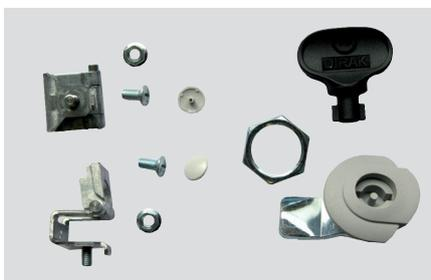
The faceplates are supplied with two packs of accessories. One contains two DIN rails with screws, which can be used to mount modular devices on the front panel. The other contains the hinges and screws for fixing the faceplate to the faceplate support as well as the ¼ turn lock with its adjusting nut and double bar key.
