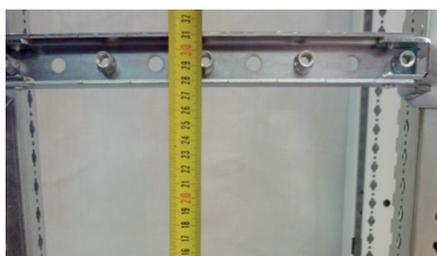
Intermediate supports are then fixed every 300 mm (tightening torque: 15 N·m).
