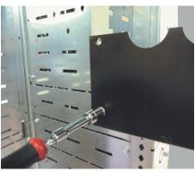
Screw in the middle panel using the eight screws supplied.
