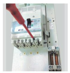
Place the device in the drawer and secure it with the two screws supplied with the circuit breaker (tightening torque  $1 \text{ N} \cdot \text{m}$ ).
