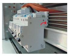
Position the circuit breaker on the rail by first pushing in the bottom of the appliance, then exerting pressure on the top to push the circuit breaker into position. The product is then automatically connected to the distribution block.
