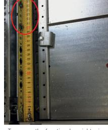
To secure the functional uprights, insert the clip-nuts 200 and 250 mm from the front.
