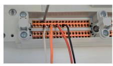
Connect the wires to the module for auxiliary circuits on the movable part of the base. The connection module has screwless terminals and the use of Starfix ferrules is recommended for wiring.
