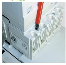
Place the appliance on the base, then secure it with the screws supplied with the circuit breaker (tightening torque 1 N·m).
