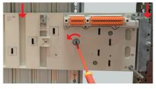
Check that the base is in the correct position by applying gentle downward pressure and then lock the ¼ turn screw to hold the base in position.
