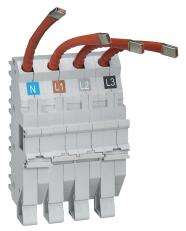
Pre-wired bases require a specific order of operations when mounting DX³ MCBs. To prevent any risk of contact with live parts, the wires must be connected to the circuit breaker before installing the base on the distribution block.
