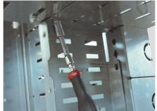
Insert the kit in the side partitioning slot of the chassis, then secure it with the six screws supplied.
