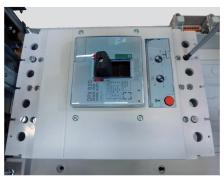
Fix it using the four screws supplied with the circuit breaker (tightening torque: 1 N.ml
