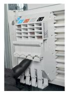
Complete installation of the support base by closing the locking levers.
