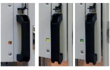
The three tray positions: "inserted", "test", "removed", are indicated with a coloured LED
