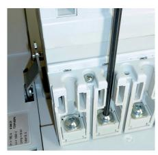
Tighten the upstream and downstream electrical connections with the eight (or six) screws provided with the base (tightening torque: 7N-m -> DPX<sup>3</sup> 160; 10N-m -> DPX<sup>3</sup> 250; 24N-m -> DPX<sup>3</sup> 630).
