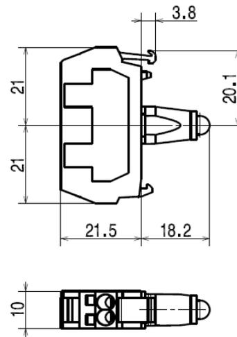
Blocs led raccordement faston
