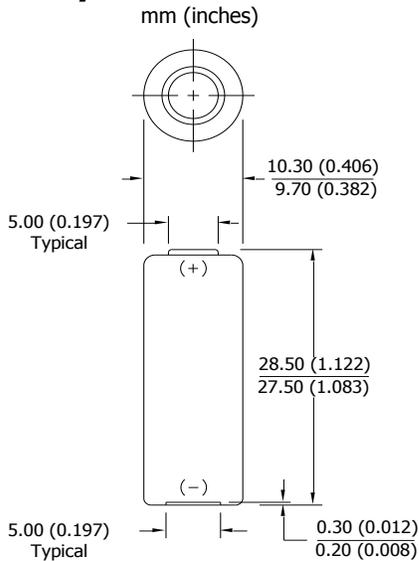
Designed for electronic applications which may require high rate pulses.
