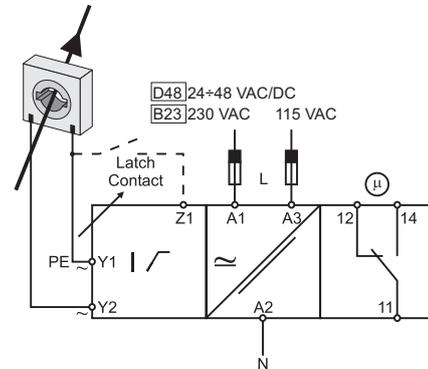
**Fig. 4** Connection by standard CT
