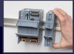
DIN rail footprint reduced by ~ 25%. Single, reliable bus connection system for both SMs and CMs.
