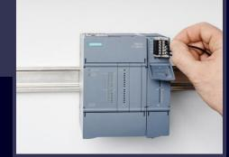
Removable high(er) density terminal blocks with push-in wiring for ease of use  $\rightarrow$  non-contact pre-wiring position.
